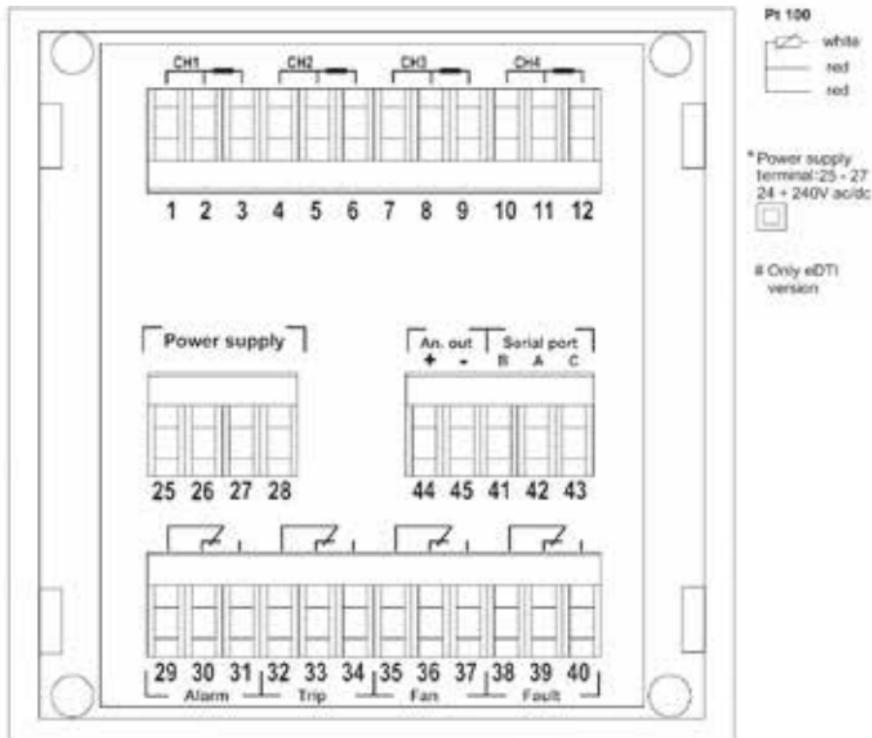
View rear panel of the instrument with terminals for the connections
