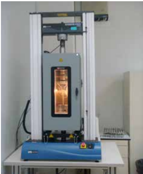
Universal Test Machine (50 kN) Environmental Chamber Test Temperature: Between Ambient Temperature & +350°C
